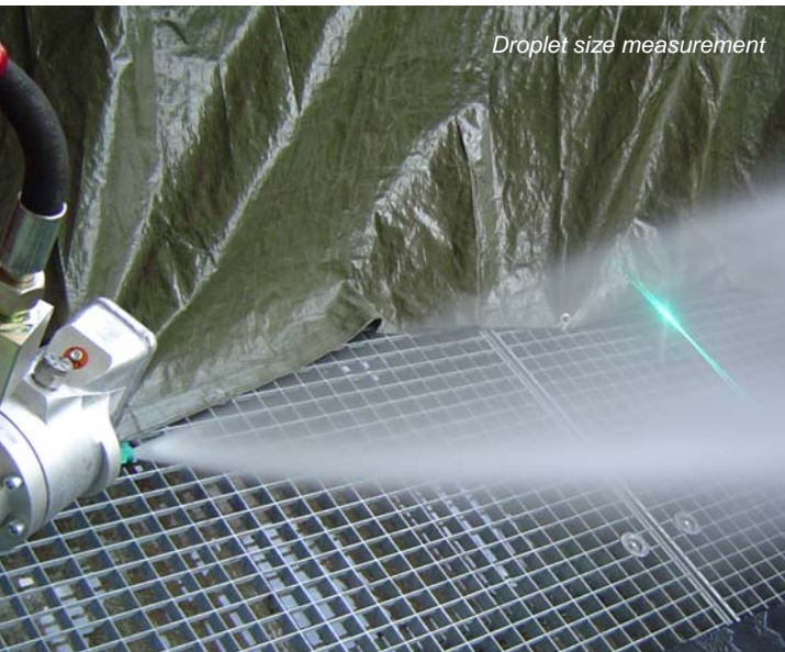
Snowmaking in the climate controlled wind tunnel of the ITFE
